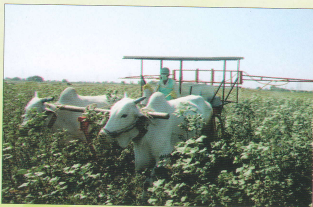
Fig. 5: Spraying operation on cotton crop using bullock drawn solar powered high clearance sprayer
