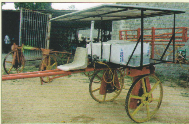
Fig. 3: A view of bullock drawn solar powered high clearance sprayer
