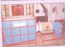
dryer of 125-500 kg capacity. Both raw and parboiled paddy can be dried in this dryer. Drying is accomplished on thin layer principle. The air temperature can be maintained at  $40 \pm 2$ °C throughout the drying period. Paddy at moisture content of 20% was dried to 14% in 6-7 hrs using 10 kg of coal in the furnace. Cost of the
