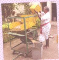
CRRI Power Rice Winnower cum Cleaner is a power operated machine to clean threshed paddy crop. Its capacity is 500 kg/hr of clean paddy, having cleaning efficiency of 99%. Cost of the machine is Rs.18,000.
