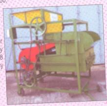
CRRI Mini Paddy Parboiling Unit is a small size parboiling unit to produce quality parboiled rice by employing improved process. The process involves soaking the paddy at 75 °C for 3.5 hrs followed by open steaming for 30-45 minutes. The process ensures uniform parboiling, without any bad smell and produces light coloured rice with better consumer preference. It takes 5-6 hours to parboil 75 kg of paddy in one batch. Cost of the machine is Rs. 5,500.
