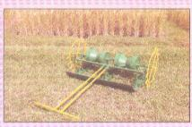
CRRI Six row manual drum seeder (Cylindrical shape) is suitable for sowing of sprouted paddy seed in puddled field at row spacing of 20 cm. Its field capacity is 0.037-0.04 hectare per hour. Its unit cost is Rs. 6500. It reduced seed rate by 35-40% as compared to broadcast seeding and reduced weeding cost about 55%.
