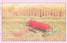
CRRI eight row self propelled seeder is an eight row, engine operated paddy seeder. It is suitable for sowing of sprouted paddy seed in puddled field at row spacing of 20 cm. Its field capacity is 0.23-0.25 hectare per hour. Its unit cost is Rs. 60,000. Pre-germinated paddy seeding has economical and operational advantages over traditional planting methods because it eliminates nursery raising, transportation and physical damage to the seedlings.
