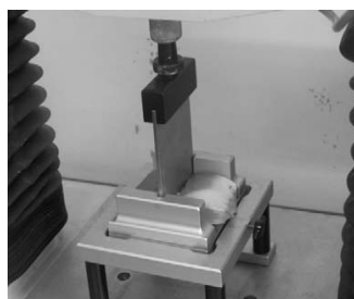
Fig.3. Cutting test of Aloe vera leaf sample
