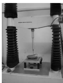
Fig. 2. Penetration test of Aloe vera leaf sample
