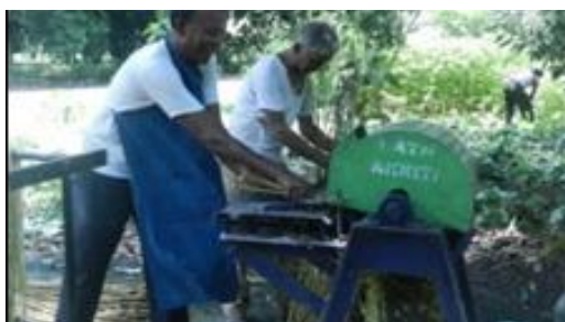
CRIJAF Ramie & Sisal Fibre Extractor
