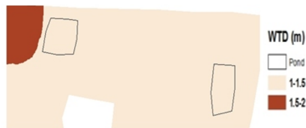
Fig. 3d. Spatial map of water table depth in post monsoon season in 2015 at Nain farm
