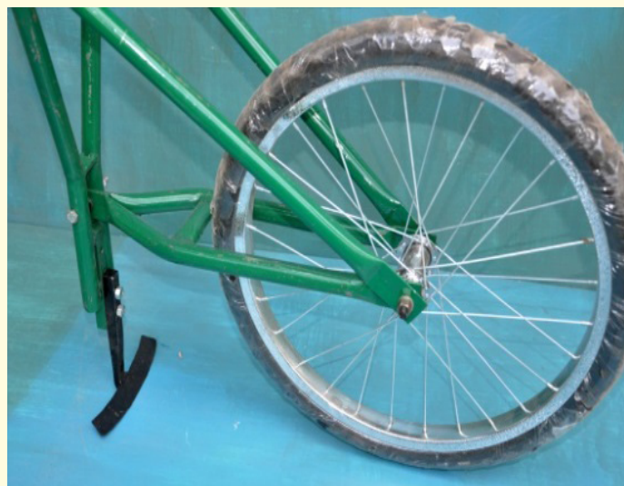
CRIJAF single wheel jute weeder with modified scraper
