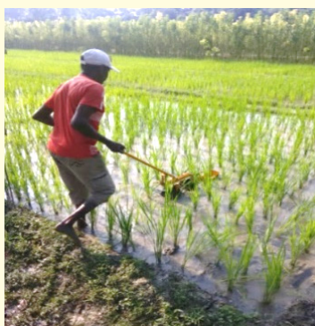
CRIJAF Jute- Paddy weeder and its operation in transplanted rice
