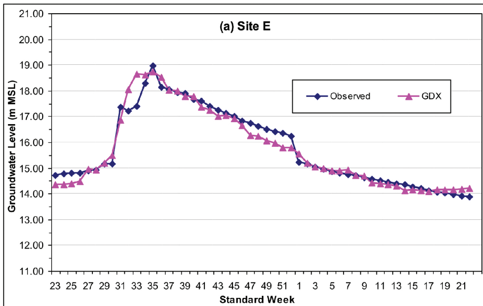
Fig. 9 (a): Comparison between observed and predicted groundwater levels at site E during testing period.
