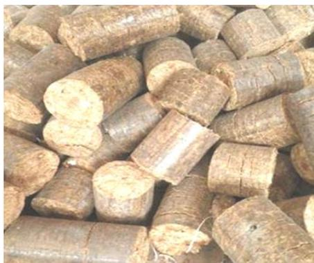
**Fig. 6: Cotton Stalk briquettes**
