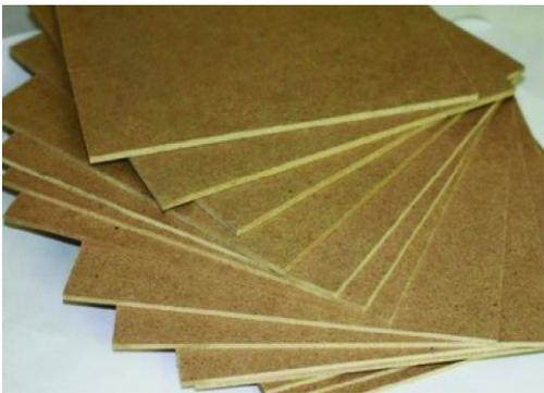
**Fig.12: Cotton stalk particle boards**
