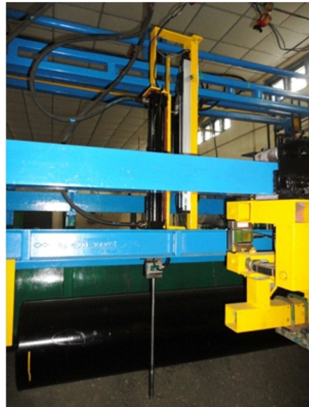
Fig 2: Hydraulically operated instrumented cone penetrometer
