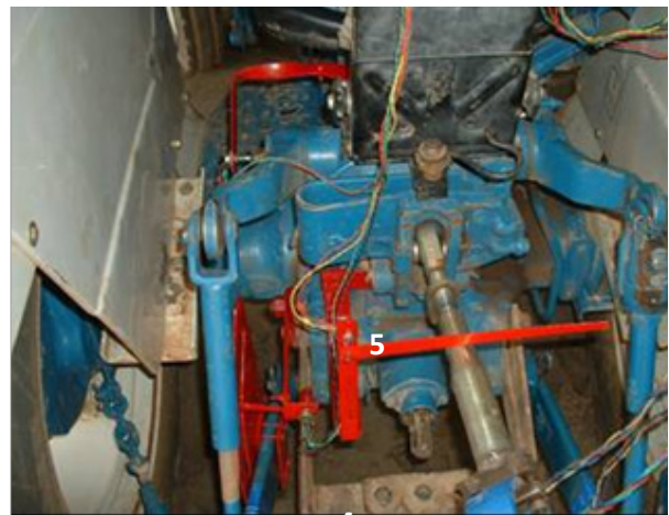
1. Top link 2. Lower link 3. Lower link vertical angle 4. Lower link horizontal angle 5. Top link vertical angle
