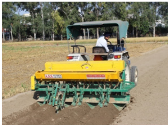
Fig. 1: Operational view of bed planter
