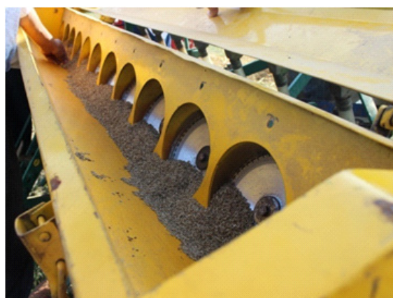
Fig. 2: View of inclined plate mechanism of mechanical bed planter
