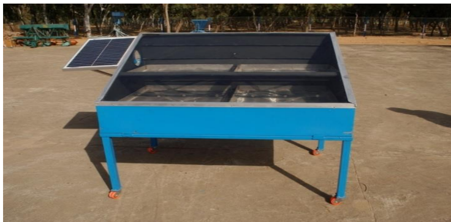
Figure 4: PVT hybrid solar dryer installed at CAZRI solar yard
