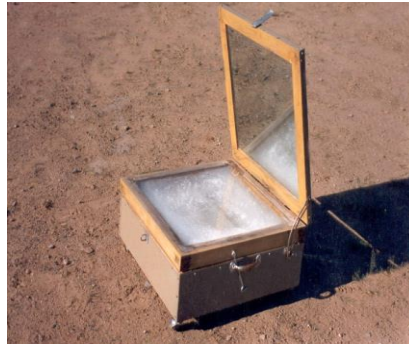
Figure 4: hot box solar cooker with transparent insulation material (TIM)
