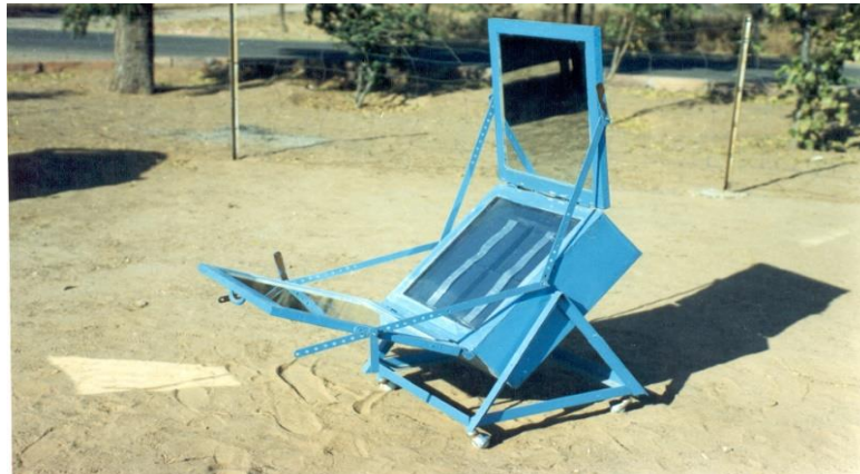
Figure 3: improved hot box solar cooker with tilted absorber
