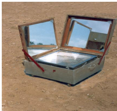
Figure 5: Double reflector hot box solar cooker with a transparent insulation material (TIM)
