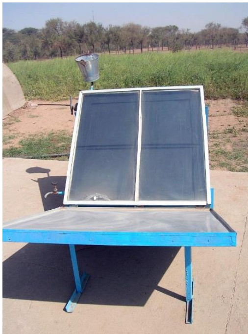
Fig. 6. Collector cum storage type solar water heater
