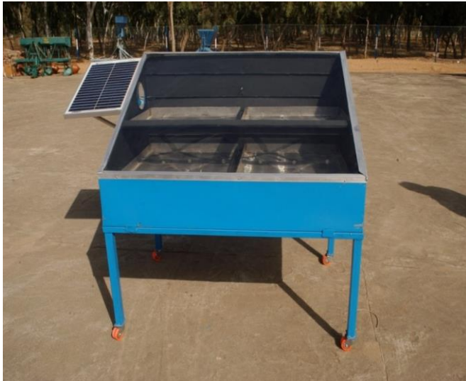
Fig. 3. PVT hybrid solar dryer installed at CAZRI solar yard
