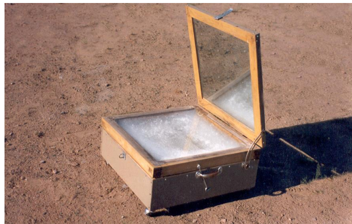
Fig. 6. Hot Box Solar Cooker with Transparent Insulation Material (TIM)
