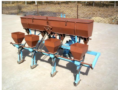
Fig. 6. Modified seed drill for inter row cropping
