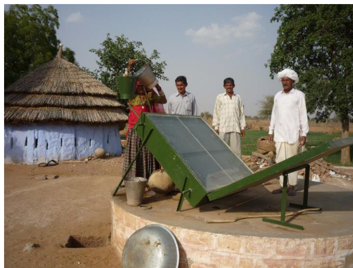
Fig. 2. Integrated collector storage solar water heater at village Newara Road Solar Dryer
