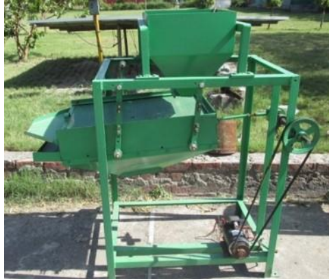
Fig. 5. Solar powered screen cleaner
