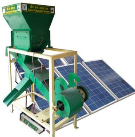
Fig. 4. Solar powered pneumatic grain/seed cleaner
