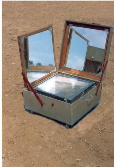
Fig. 7. Double Reflector Hot Box Solar Cooker with a Transparent Insulation Material (TIM)
