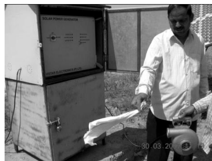
Fig. 3. Operation of pump and blower by PV generator
