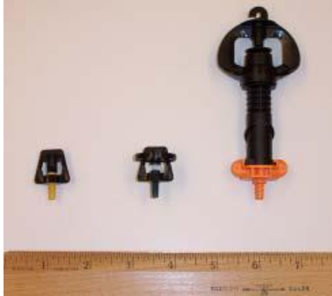
Fig. 3. Micro sprinklers of different sizes
