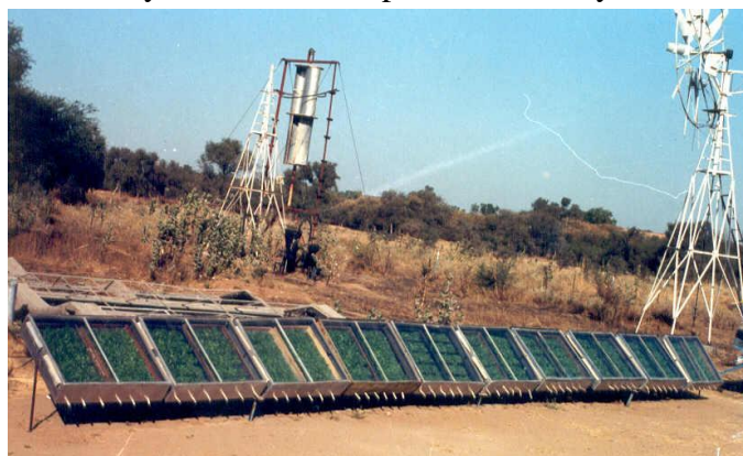
Fig. 13. Commercial Solar Dryer with Inclined Surface
