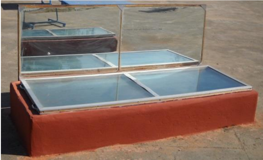
Fig. 2. Improved solar cooker for animal feed installed in the field
