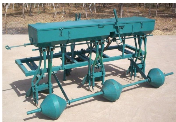
Fig. 3. Tractor operated six rows (three furrows) seed cum fertilizer drill for sowing on slanting surfaces of a furrow
