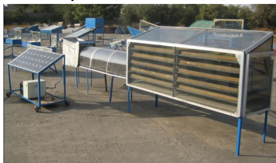
Fig. 7. PV winnower cum dryer with pre air heating tunnel
