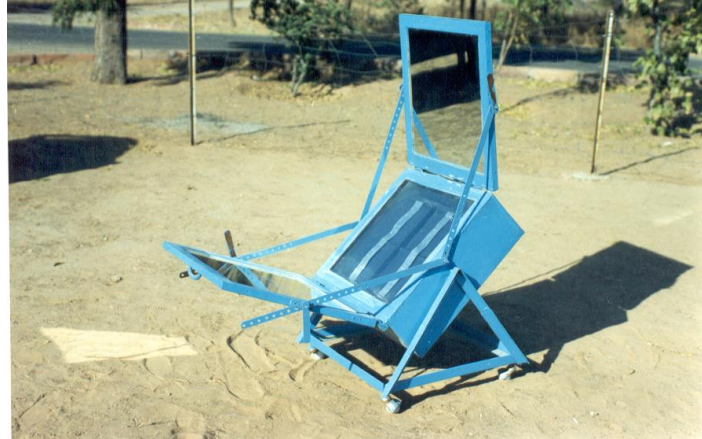
Fig. 5. Improved Hot Box Solar Cooker with Tilted Absorber
