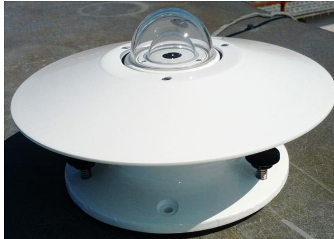
Fig.1. A photograph of a typical pyranometer
