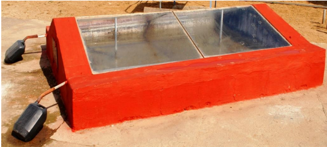
Figure 3: Solar desalination devices made of vermiculite-cement plastered material
