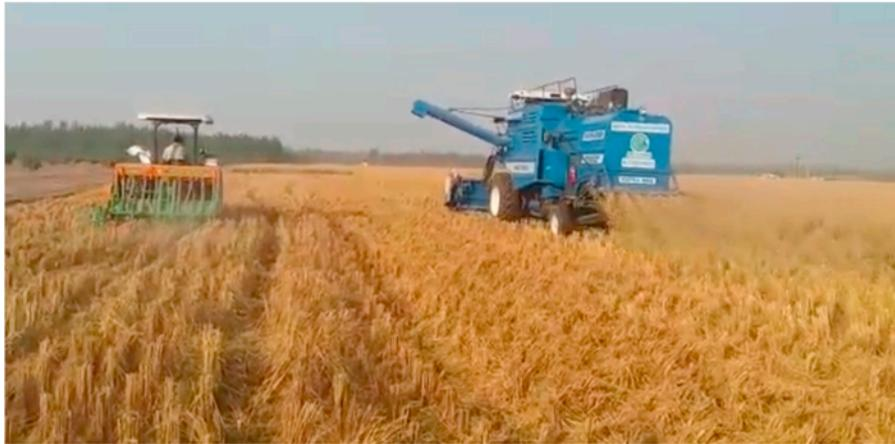
Fig. 7. A view of super straw management system attached behind the combine harvester and direct drilling of wheat seed by happy seeder.
