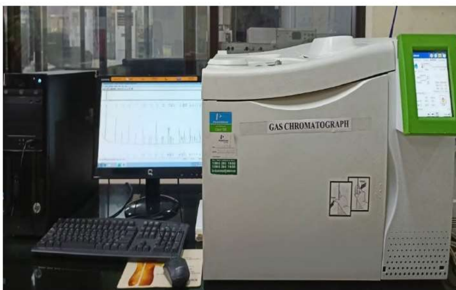
Figure 3: Perkin Elmer Clarus 580- Gas chromatograph -FID
