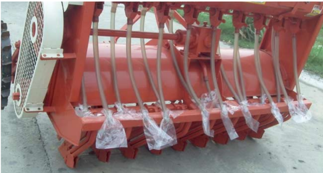
Figure 21. Seed and Fertilizer calibration in laboratory
