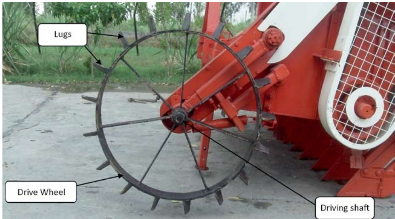
Figure 16. Drive wheel and components
