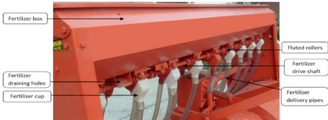
Figure 12. Fertilizer metering system
