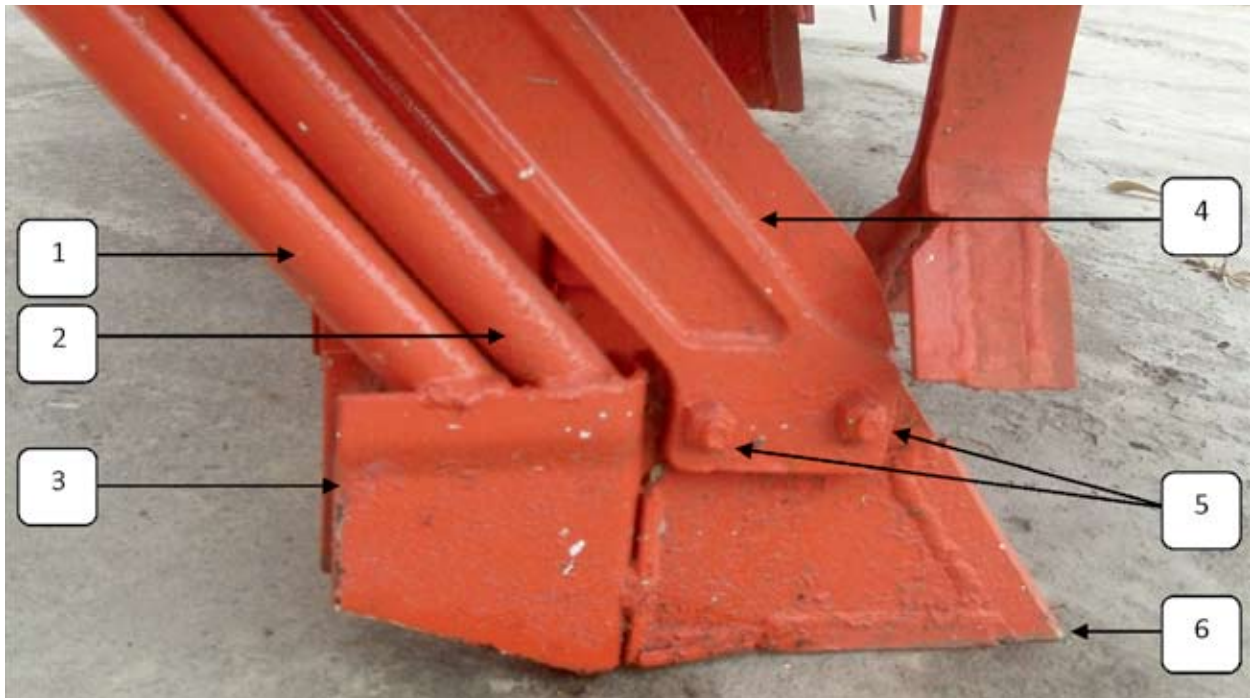
Figure 2. Major parts of furrow opener/slit
