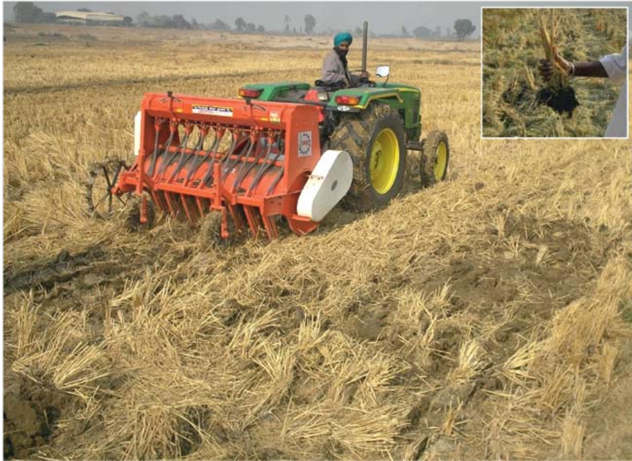
Figure 27. Uprooting of anchored rice residues due to high soil moisture content.
