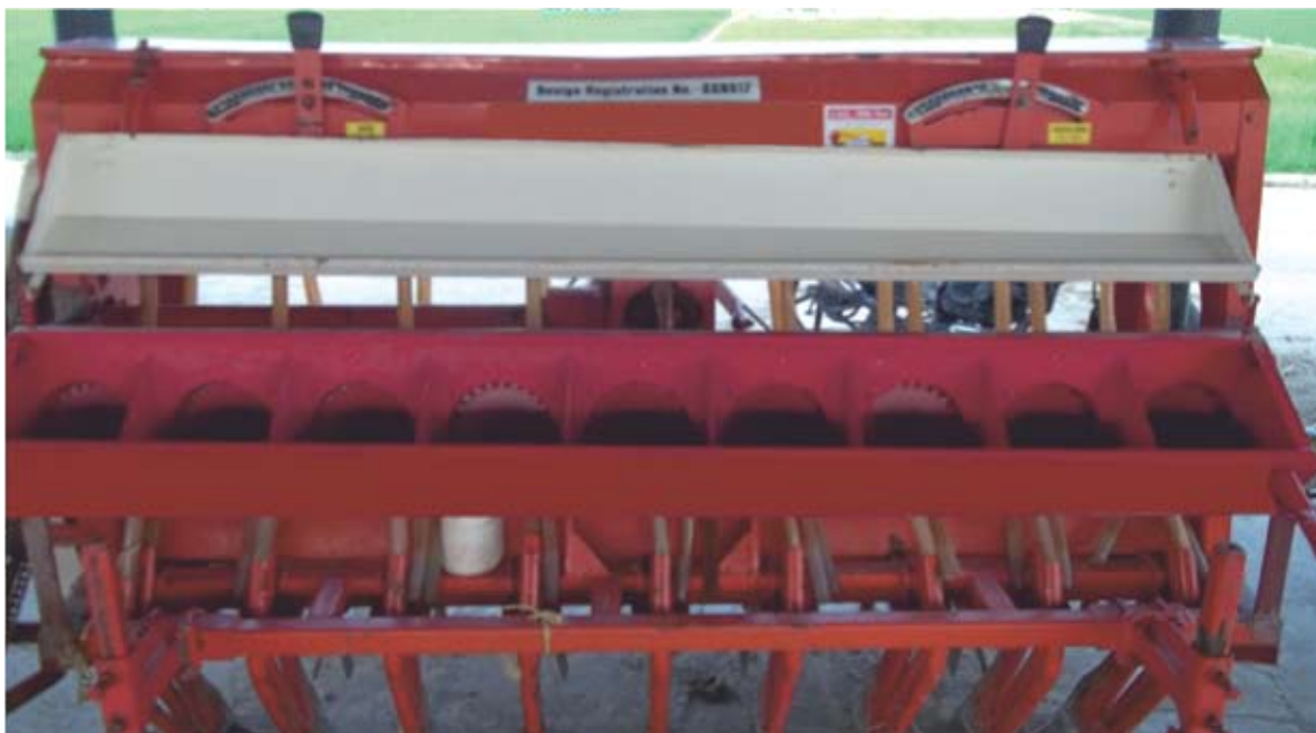
Figure 6. Modified seed box of turbo happy seeder
