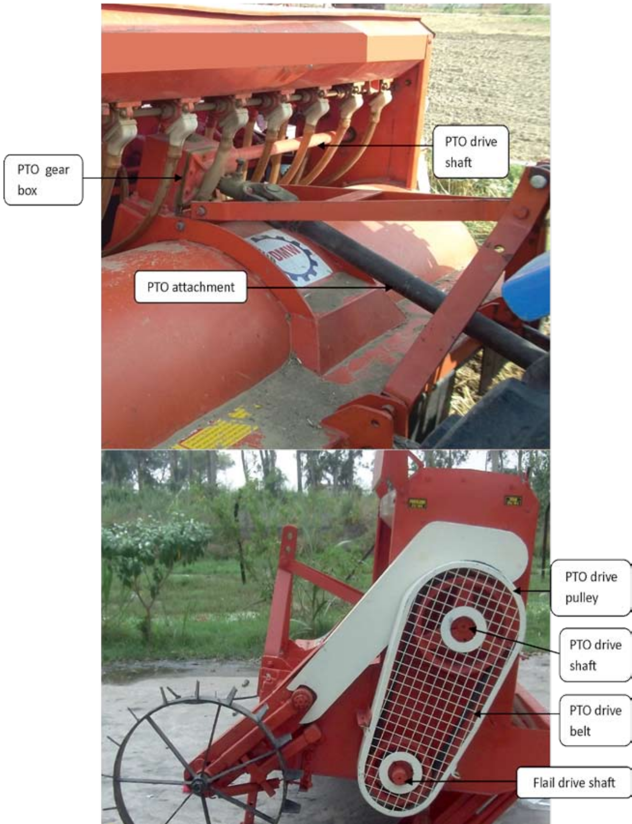
Figure 18. Power transmission system by PTO shaft
