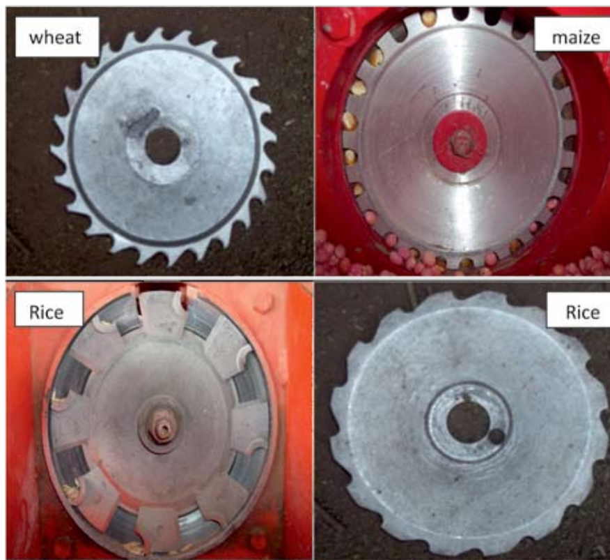
Figure 11. Types of inclined plates used in modified THS
