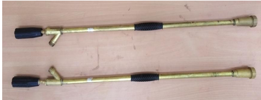
Fig. 2. ASPEE SPGF-80 cm spray guns used for the experiment
