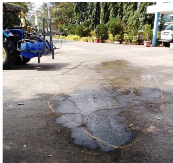
Fig. 3. Marking of wetted perimeter for left spray gun
