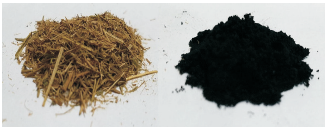
Biochar production using rice stubble
