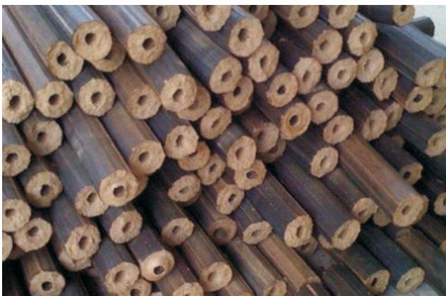
Rice straw briquette and straw pellet
