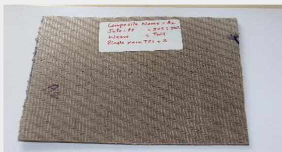
Jute reinforced Polypropylene Composite
