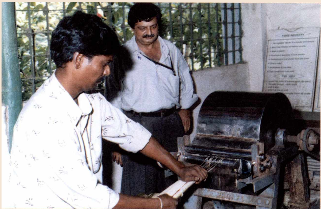
Banana fibres being extracted from the modified Raspador Fibre Extractor
