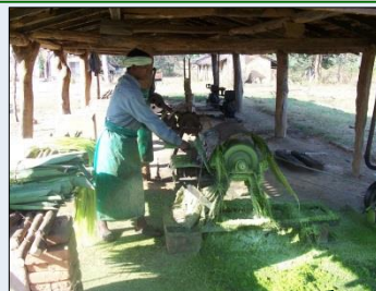
Extraction Fibre from sisal leaf
