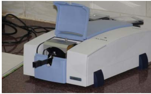
Fig. 2. FT-MIR spectrometer and MIR Absorption Spectra
