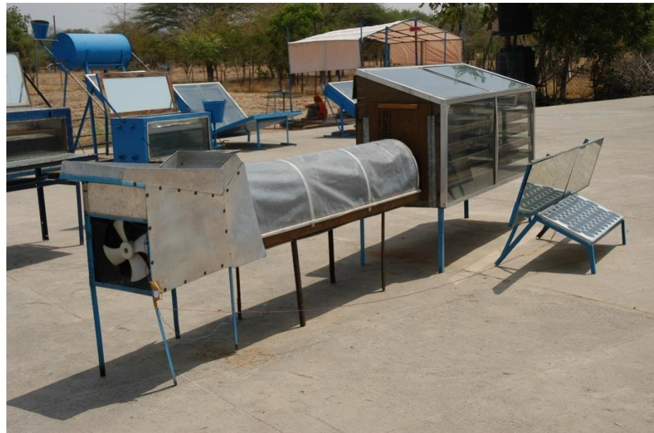
Figure 3. Picture depicting the installation of the PV/T hybrid solar dryer with a winnower at the CAZRI solar yard in India.
