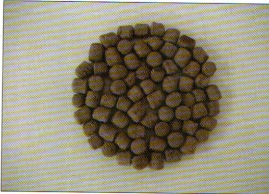
Extruder feed pellets with oil coating
