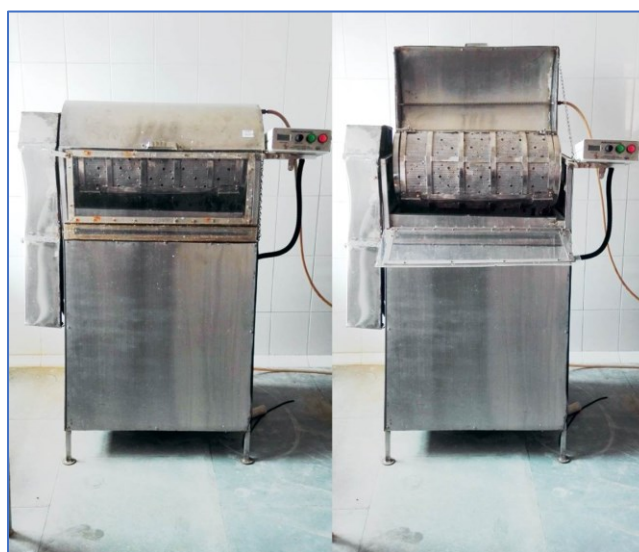
Fig. 5. Fish de-scaling machine with variable drum speed
