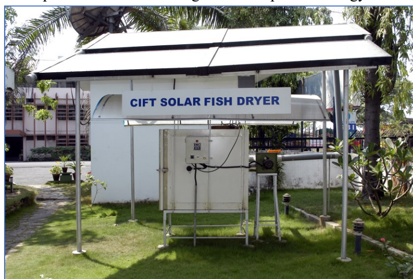
Fig. 2. ICAR-CIFT Solar-electrical hybrid dryer
