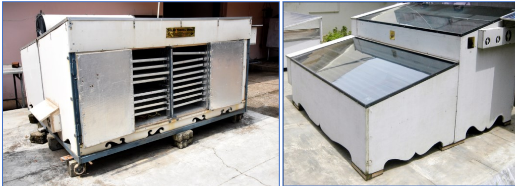
Fig. 3. ICAR-CIFT Solar-electrical hybrid dryer
