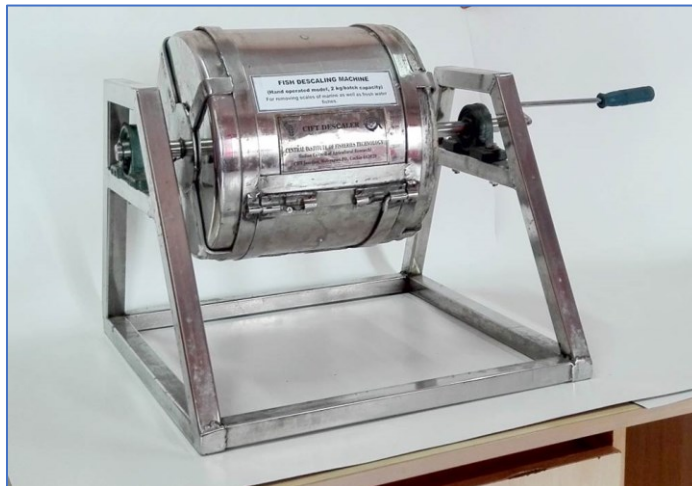
Fig. 7. Hand-operated fish de-scaling machine
