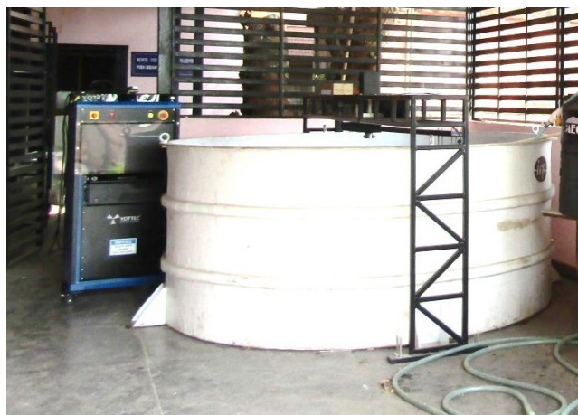
Fig. 4 Moving gantry system installed at ICAR-CIFT for studying swimming speed of fish
