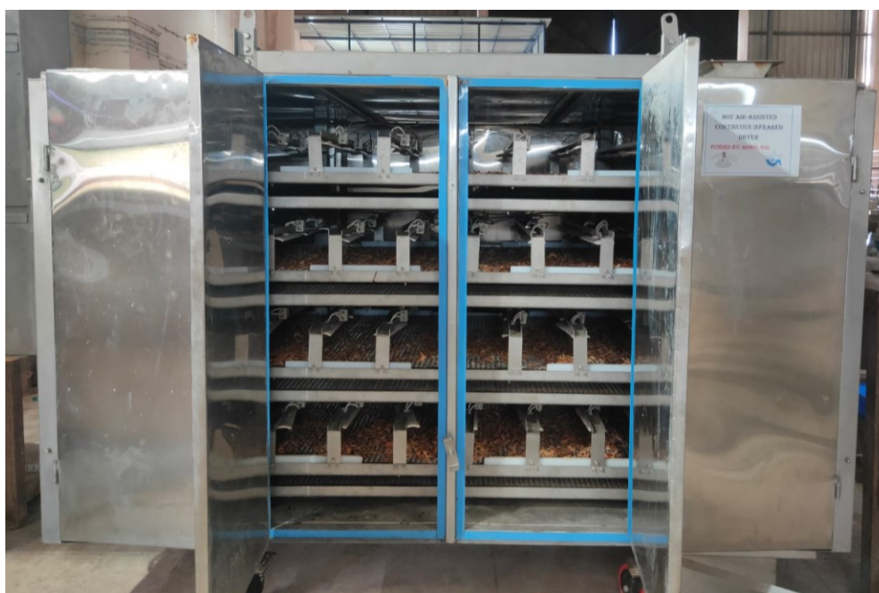
Fig. 1 Pilot-scale hot air-assisted continuous infrared dryer
