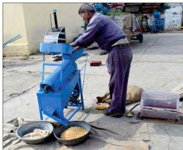
Final Prototype of VL Maize sheller under operation
