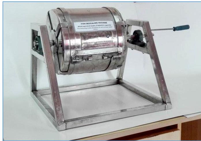
Fig. 7. Hand operated fish de-scaling machine
