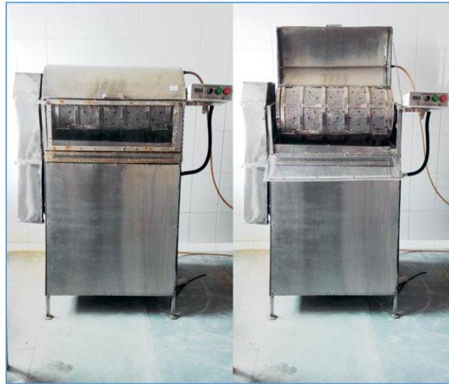
Fig. 5. Fish de-scaling machine with variable drum speed
