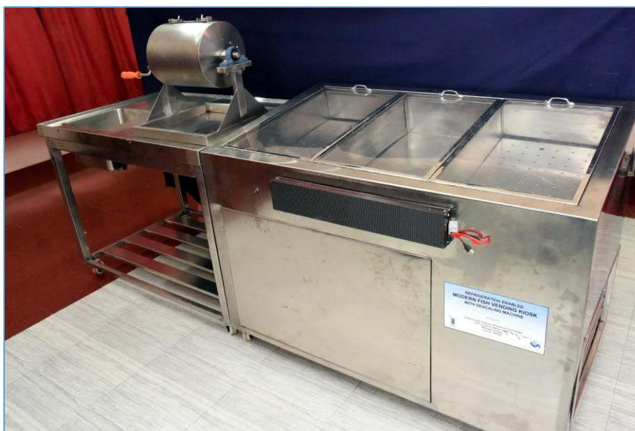
Fig. 8. Refrigerated mobile fish vending kiosk
