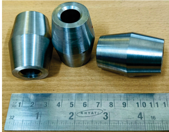
Fig.5 Prototype of stainless steel sinkers made for bottom trawls
