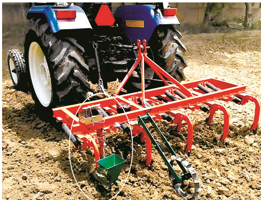
Fig. 5 — Field evaluation of electronic seed metering system retrofitted on a cultivator frame.
