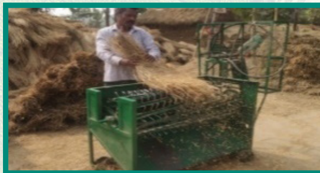
Operation of power operated thresher-cum-winnower
