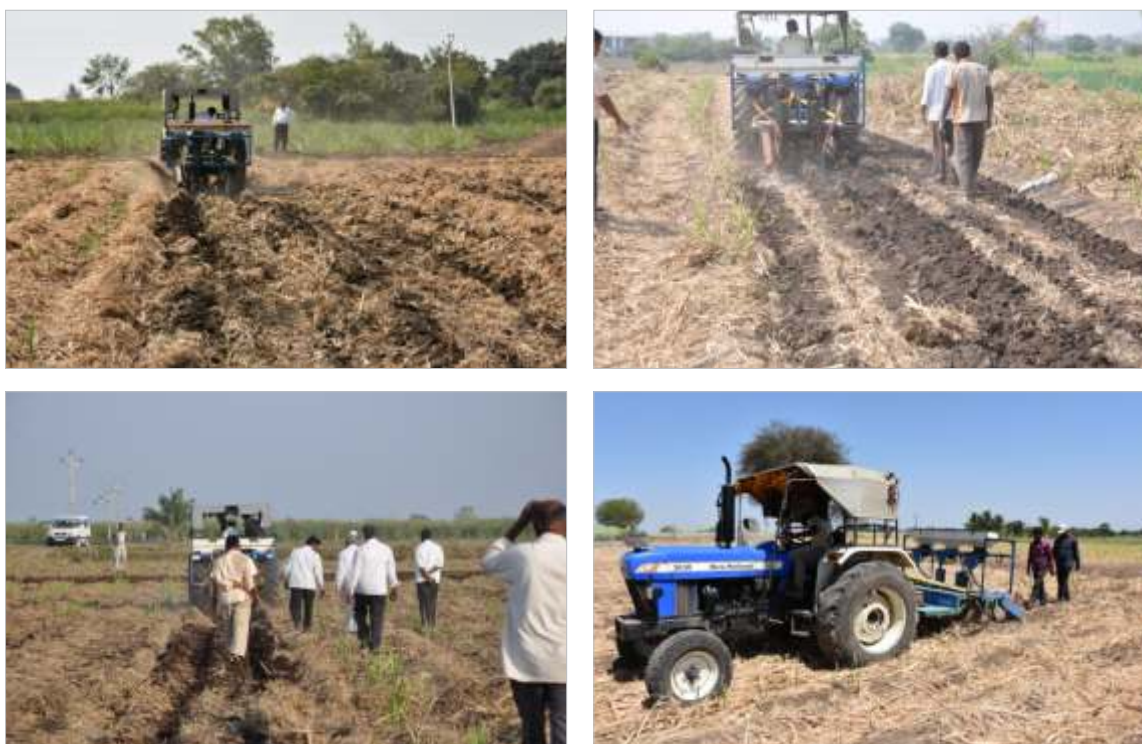
Fig. 2.34. Demonstration of stubble shaver, off-bar, root pruner cum fertilizer drill (SORF) machine at farmer's fields.
