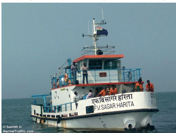
F V Sagar Haritha (LOA 19.75m, fuel efficient multipurpose fishing vessel)
