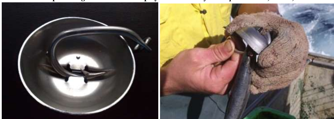
The shield gets fitted to a baited Smart Tuna Hook. Courtesy: ACAP, 2015
