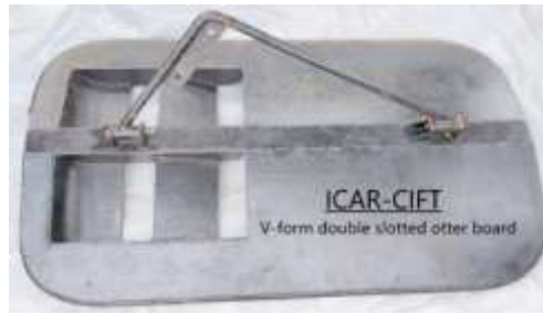
1500mmx 900mm (110kg) V-form double slotted otter board
