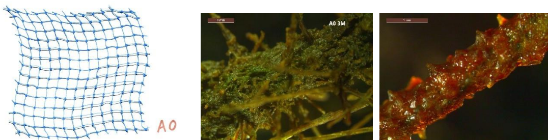
Fig 1. A) PE cage net b) PE cagenet after 3 months c) PE cagenet treated with PANI+nano CuO after three months exposure in the estuary.
