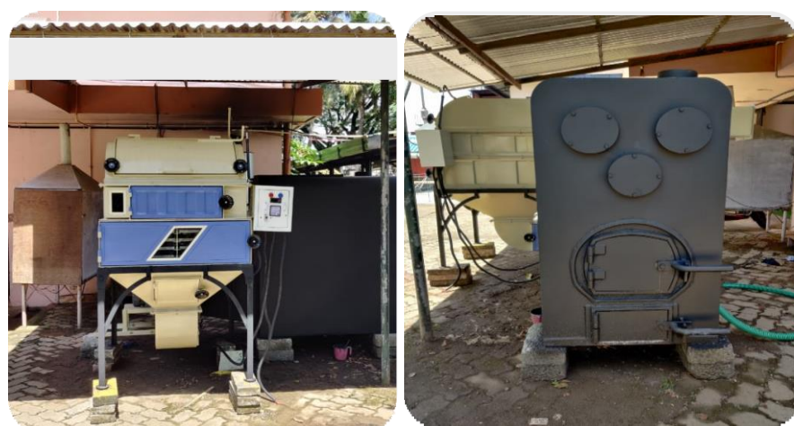
Fig. 6. ICAR-CIFT Biomass dryer
