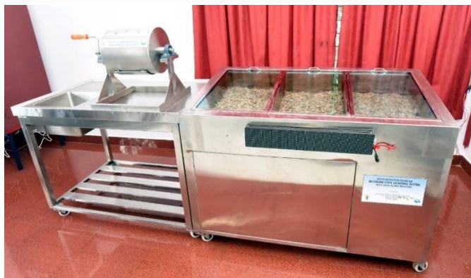
Fig. 15. Refrigerated mobile fish vending Kiosk
