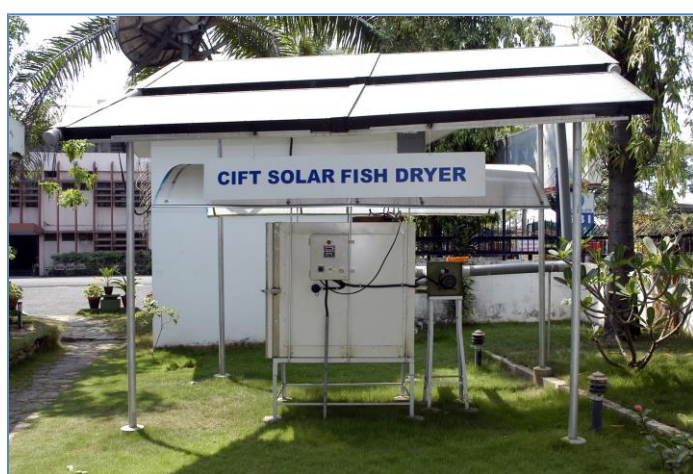
Fig. 3. ICAR-CIFT Solar-electrical hybrid dryer
