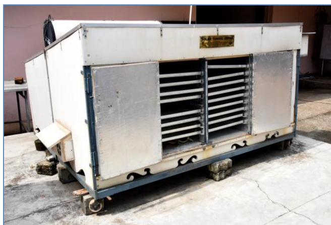
Fig. 4. ICAR-CIFT Solar-electrical hybrid dryer
