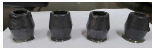
Fig. 6. Abrasion test data of 0.5% SiO 2 reinforced bisphenol A epoxy polymer coated lead in two different thickness after 1000 cycles of operation in abrasion tester. b) composite coated arranged in the abrasion tester drum. c) nano SiO 2 – epoxy polymer coated lead sinkers.
