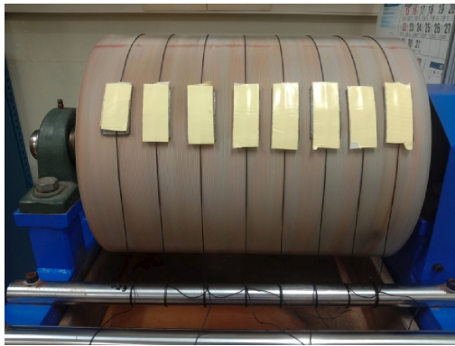
Fig. 6. Abrasion test data of 0.5% SiO 2 reinforced bisphenol A epoxy polymer coated lead in two different thickness after 1000 cycles of operation in abrasion tester. b) composite coated arranged in the abrasion tester drum. c) nano SiO 2 – epoxy polymer coated lead sinkers.
