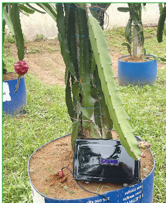
Fig. 2 Display of Volumetric Soil Moisture content in the LCD and Android based Mobile app (Ajit Kumar Nayak, S. Pradhan, A. Sarangi, S.K. Rautaray, J.S Bal and N.M. Jeepta)
