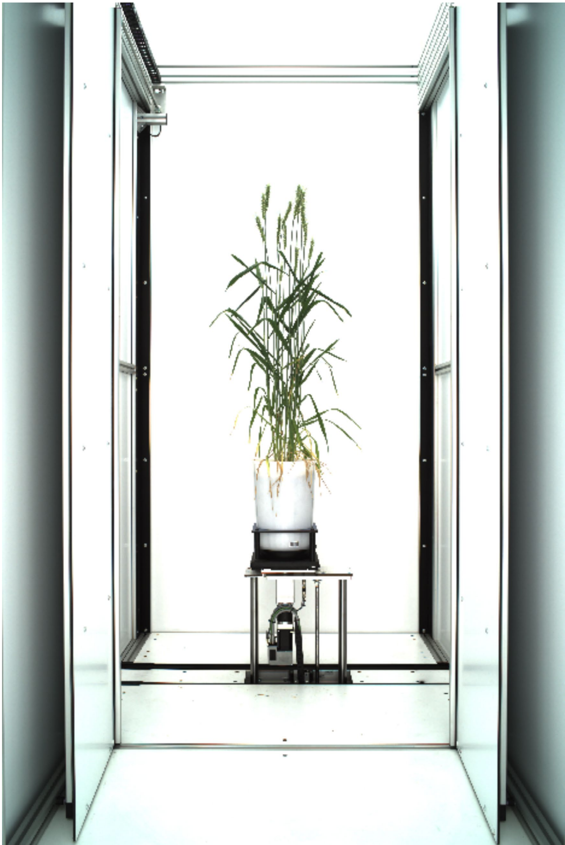
Fig. 1 Imaging chamber and the captured image of wheat plant in NDPPC facility
