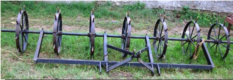
Fig. 5. Tractor-drawn hole making implement for sowing
