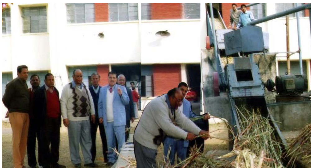
Image 1. Sweet sorghum pilot study: Sweet Sorghum cane being put in the cane carrier and Prof GK Shukla, Director, NSI , Kanpur and other faculty are overseeing the crushing process ( Shukla et al 2006)
