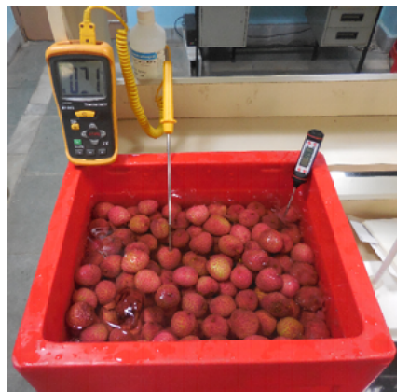
Temperature reduction through hydro-cooling
