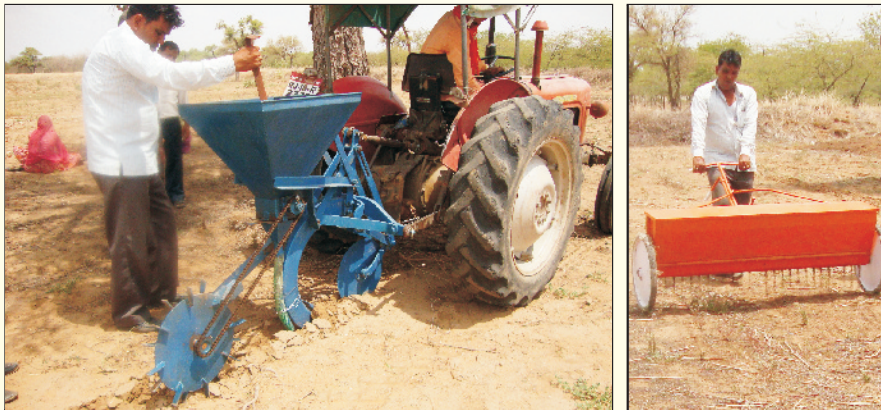
Fig. 28. Prototypes of surface and subsurface manure applicators.
