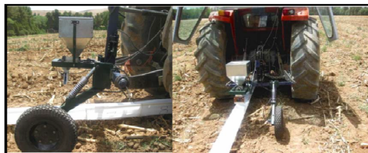
Fig.6. Two views showing the components of ground-driven wheel used for measurement of tractor travel speed and displacement (Forouzanmehr and Loghavi., 2012)
