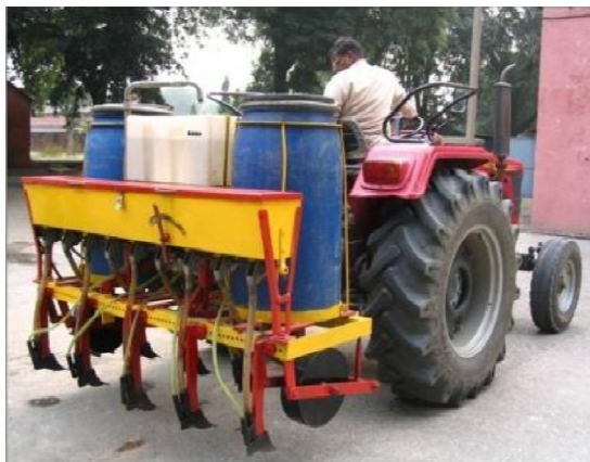
Fig. 1. Pusa Aqua-ferti-seed-drill machine mounted on tractor
