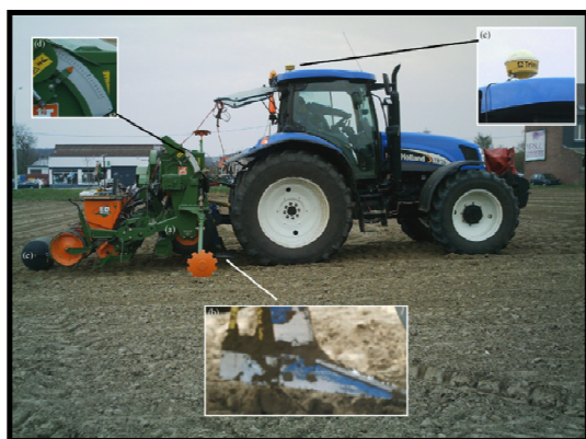
Fig.3. Developed soil sensor based variable rate Phosphorus applicator (Source: Maleki et al. , 2008)
