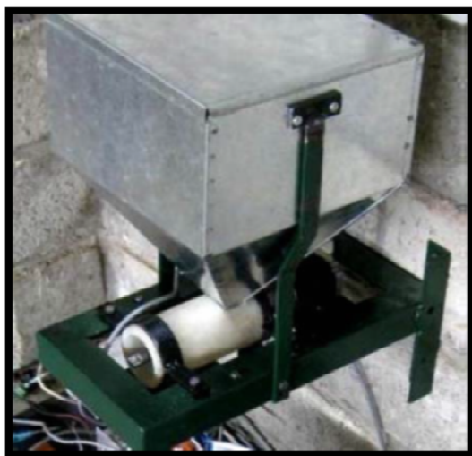
Fig.4. Fertilizer hopper and metering screw assembly used for laboratory and field tests(Forouzanmehr and Loghavi., 2012)
