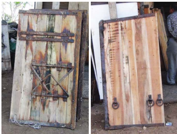
Fig. 1. Dorsal and ventral view of traditional rectangular flat wooden otter boards of Veraval coast
