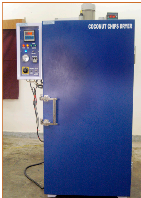
Fig. 13a Electrical dryer
