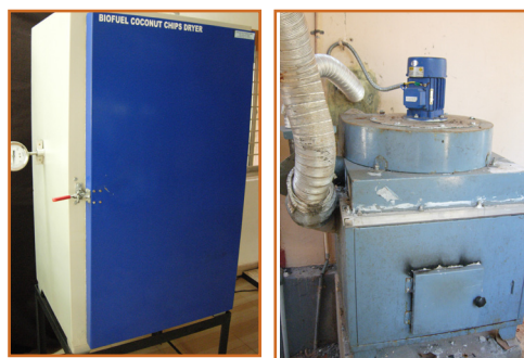
Fig. 14 Biofuel dryer for coconut chips drying (Drying chamber & Heating chamber)
