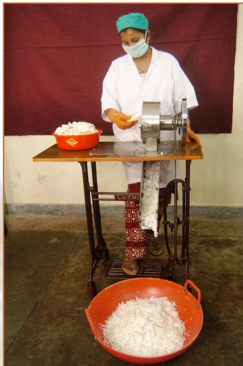
Fig. 9 Sewing machine based coconut slicer
