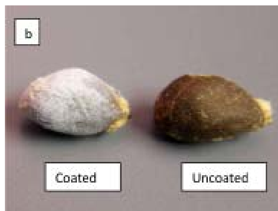
Seeds of coated and uncoated wheat (a) & coated and uncoated cotton (b) by electro-spinning
