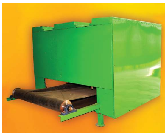
NIRJAFT Power Ribboner Machine for Extraction of Fibres from Jute & Mesta Plants
