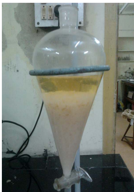
Fig. 1 - Extraction of dhaincha solvent gum extraction
