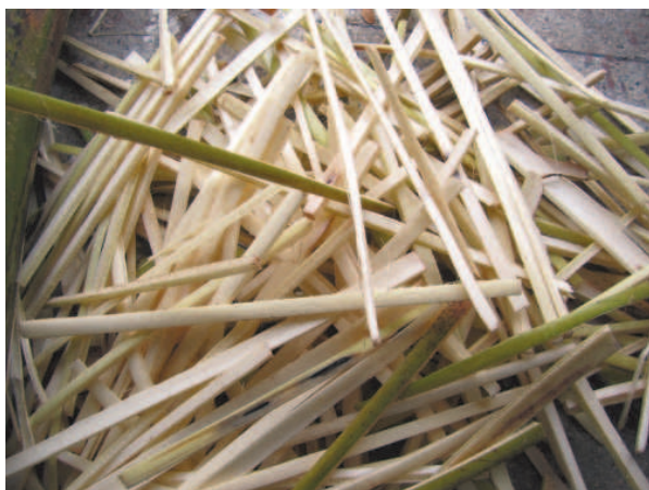
Figure 1. Shredded pseudo stem for retting
