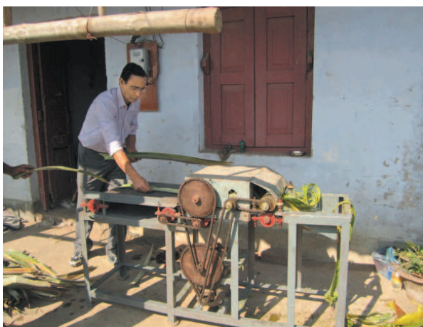
Figure 2 : Scratching of Pineapple Leaf
